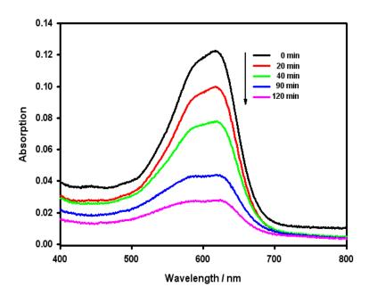
Fig. 4- Time-dependent absorption spectra of the M5B solution with initial concentration of 6.1 mg/L under UV-vis irradiation and using nano-composite copper-zinc oxide (NCCZO) coated on glass fabricated via sol-gel and doctor blade route using copper acetylacetonate,  $Cu(CH_3COCHCOCH_3)_2$  and zinc acetylacetonate,  $Zn(CH_3COCHCOCH_3)_2$  as precursors with mol ratio 1:2 annealed at 650 °C
