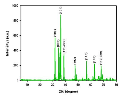
Fig. 2- XRD pattern of nano-composite copper-zinc oxide (NCCZO) coating fabricated via sol-gel and doctor blade route using copper acetylacetonate,  $Cu(CH_3COCHCOCH_3)_2$  and zinc acetylacetonate,  $Zn(CH_3COCHCOCH_3)_2$  as precursors with mol ratio 1:2 annealed at 650 °C
