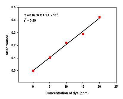
Fig. 1- Calibration curve of M5B dye concentration versus absorbance
