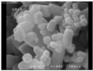
Fig. 3- FESEM image of nano-composite copper-zinc oxide (NCCZO) coating fabricated via sol-gel and doctor blade route using copper acetylacetonate, Cu(CH<sub>3</sub>COCHCOCH<sub>3</sub>)<sub>2</sub> and zinc acetylacetonate, Zn(CH<sub>3</sub>COCHCOCH<sub>3</sub>)<sub>2</sub> as precursors with mol ratio 1:2 annealed at 650 °C
