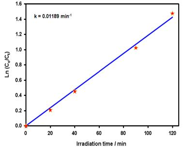
Fig. 5-  $\text{Ln}(C_0/C_t)$  vs. Time (min) for the photocatalytic degradation of the M5B dye solution under UV-vis irradiation using nano-composite copper-zinc oxide (NCCZO) coated on glass fabricated via sol-gel and doctor blade route using copper acetylacetonate,  $\text{Cu}(\text{CH}_3\text{COCHCOCH}_3)_2$  and zinc acetylacetonate,  $\text{Zn}(\text{CH}_3\text{COCHCOCH}_3)_2$  as precursors with mol ratio 1:2 annealed at 650 °C
