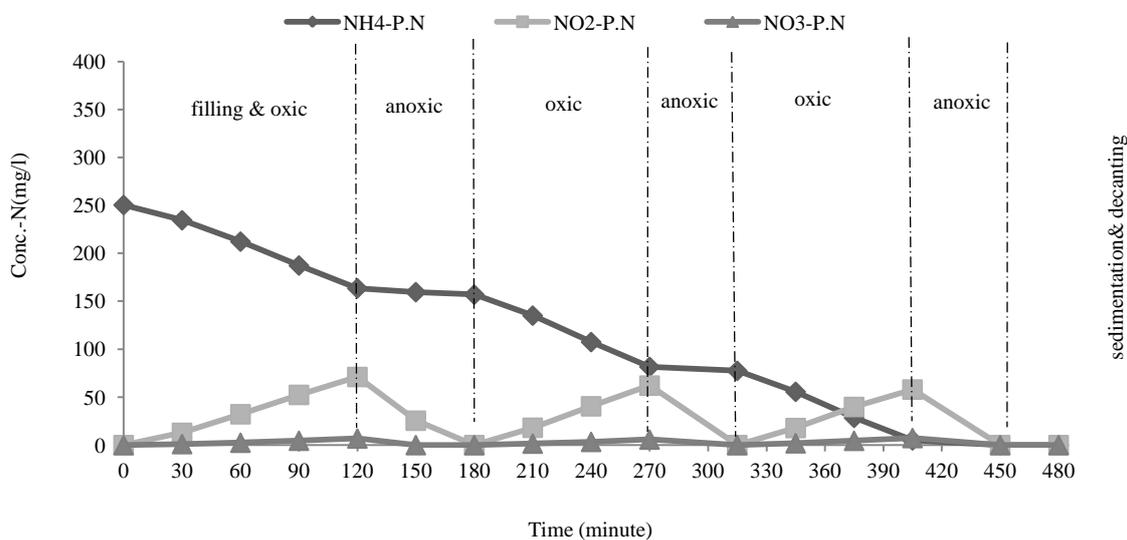
Fig. 2- Side stream partial nitrification results after steady state conditions
