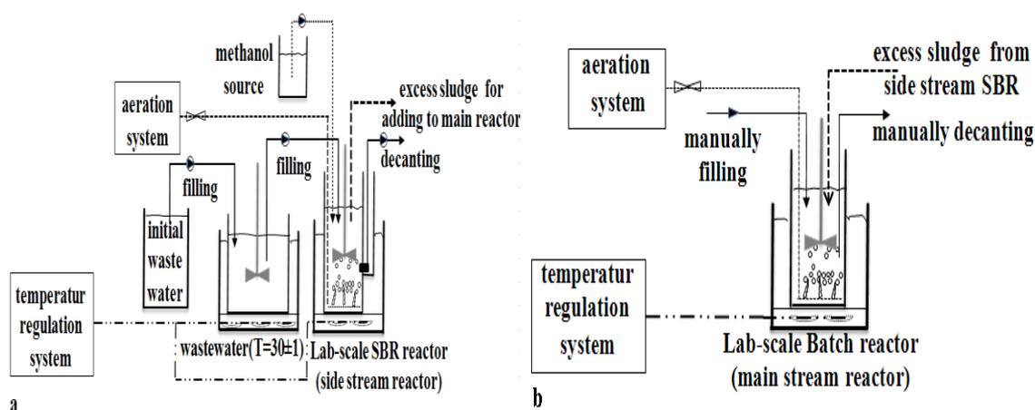
Fig. 1- a) Lab- scale side stream SBR reactor, b) Lab- scale main stream batch reactor
