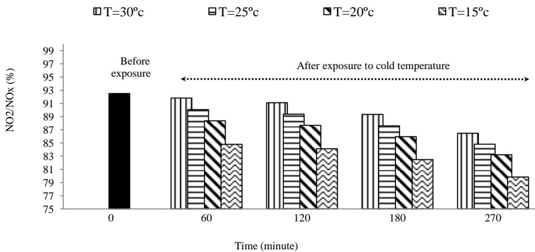
Fig. 5- Effect of temperature & time on NO<sub>2</sub>/ NO<sub>x</sub> ratio after biomass adding to new environment
