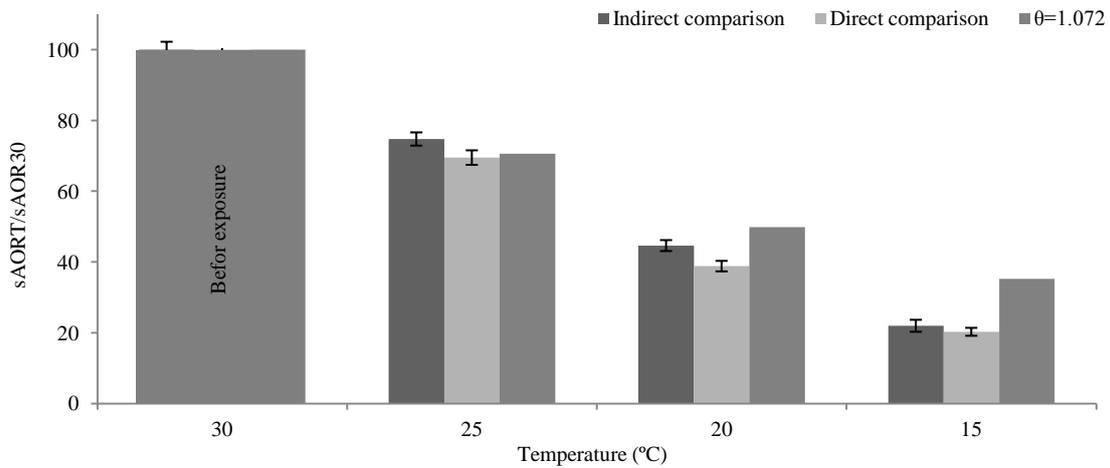
Fig. 3- sAOR reduction after cold shock in direct and indirect comparison
