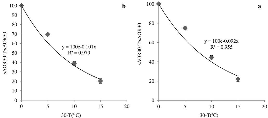
Fig. 4- Exponential trend line for temperature dependency factor calculating (a- indirect and b- direct)
