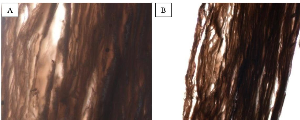
Fig.1- Multi-layer structure of vermiculite in optical microscope. a) Magnification  $\times 10$ . b) Magnification  $\times 4$ .
