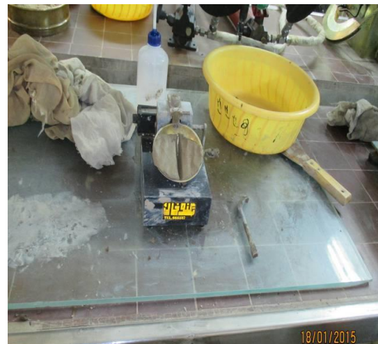
Fig. 19- View of the Atterberg Limits test (Casagrande method)
