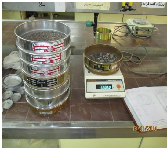
Fig. 18- View of the grain size analysis test
